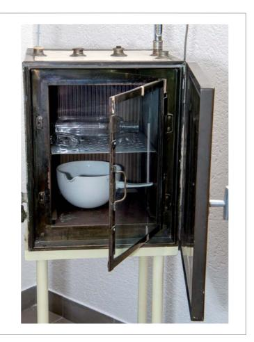
The development and growth of organisms usually require special conditions. Incubators are used to create and maintain microclimates by closely controlling conditions such as humidity and temperature. Originally, these devices were developed to hatch chicken eggs. One of the pioneers who introduced these devices into microbiological laboratory practice was Robert Koch.
