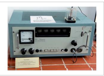
Nikolai W. Timoféeff-Ressovsky and Max Delbrück irradiated fertilized fly eggs and larvae to study the resulting mutants. To record the radioactive isotopes and interpret the results of their experiments, it was crucial to know the amount of radiation that was being used. This was the purpose of the Geiger-Müller counter.
