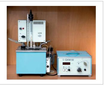
Being able to determine the concentration of glucose in liquids is crucial for research, as described above for polarimeters, and for clinical purposes such as diagnosing diabetes. The Glukometer GKM 01, exhibited here, was the first commercially available device for analysis based on a biosensor. It was developed here on the Campus Berlin-Buch.
