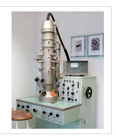
This electron microscope was made by the factory for television electronics in Berlin and dates from 1966. It has a resolution of about one nanometer. Using electronoptical and light-optical post-enlargements, it achieves a total enlargement of a factor of about one million. The first electron microscope was developed in Berlin by Ernst Ruska and built in 1933. He received the Nobel Prize in Physics for this achievement in 1986.
