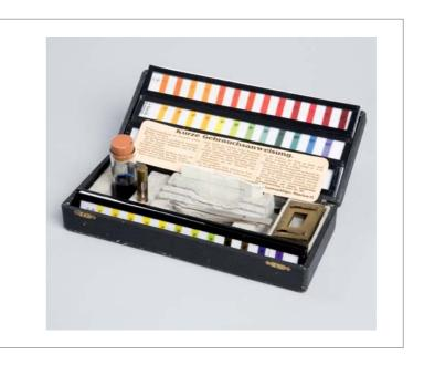
This small case contains a color test kit from the Munich company F. & M. Lautenschläger from 1900, which uses color indicators to determine the pH value of substances. This value indicates the concentration of hydrogen ions and measures how acidic or basic a liquid is. The lower the concentration of hydrogen ions in the solution, the higher the value. The pH scale runs from zero to 14. Solutions with a pH of seven are neutral; those below are acidic, and those above seven are basic or alkaline.
