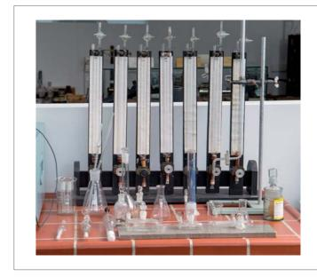
Manometers are devices that can be used to measure the pressure of a gas. In the 1920s, Otto Warburg and Erwin Negelein combined them with vessels in which biochemical reactions took place. They succeeded in determining aspects of the gas metabolism of tissues and cells – such as how much oxygen was consumed in a reaction, or how much carbon dioxide was produced. This manometric device is known as the Warburg apparatus.
