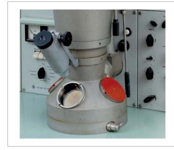
Electron microscopes achieve incomparably higher magnifications than light microscopes because they work with electron beams, which have wavelength 100,000 times smaller than that of visible light. They have become indispensable instruments for anatomical and histological studies. Subcellular structures and viruses can only be made visible with electron microscopes because light microscopes do not achieve the necessary resolution.
